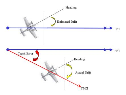
An ADF can be used to calculate your TMG from a station. Below is a diagram showing the relationship between the A/C HDG and Relative Bearing shown on the ADF. Using this information the Track Made Good can be calculated if you are tracking from an NDB. Once you know the TMG, Track Error and Actual Drift can be calculated.
