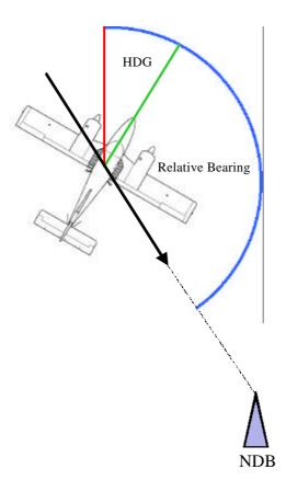
$Heading + Relative\ Bearing = Track\ TO\ Station$   $Heading + Relative\ Bearing + \text{$/$-$}180 = Track\ FROM\ Station$
